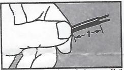
2. Hold the wire firmly approximately one inch away with the ends of insulation even.
