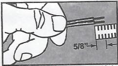
1. Cut and strip the harness wire 5/8". The correct strip length is important to ensure a good splice.
