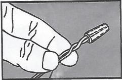
4. Inspect the finished connection by pulling on the wire connector to be sure it is secured CAUTION: DO NOT TUCK WIRES INT O THE HEATER BOX
